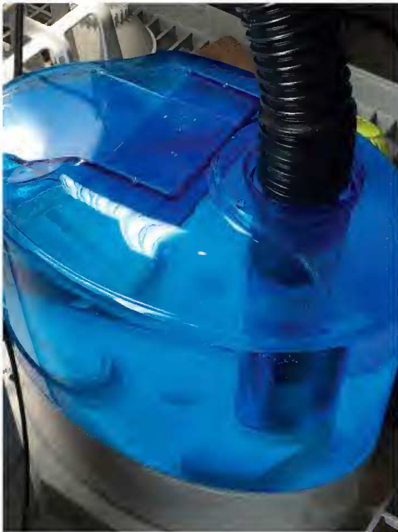
Figure 1: Ultrasonic humidifier with shop vac hose inserted into the output.
